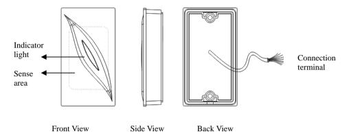
**Indicator status:** when power on, the buzzer will have a prompt sound of 'di', indicating the complete initialization, at the same time the red light will be lighted up; When brushing the card, the buzzer will have a prompt sound of 'di', at the same time the red light is off, later the green light will flash once; when in standby, the red light will be constant on. **Sense area:** sense area of card.
